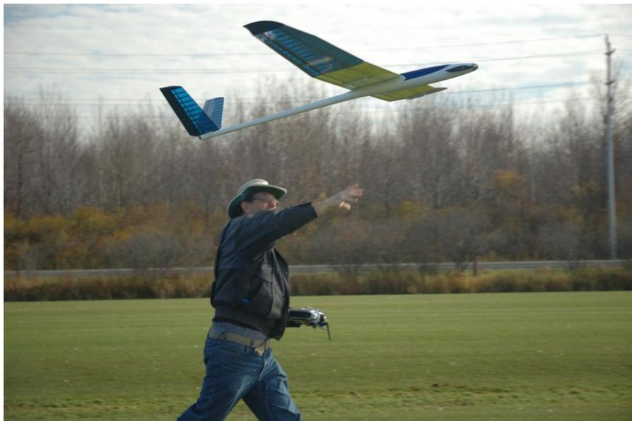
Picture #2: Aurele Alain launching his Gracia. Here, the glider is thrown with motor off and the pilot starts the motor only once it has been safely released.
